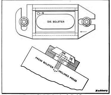
Fig. 43. Die-bed adapted to Inclined Press
